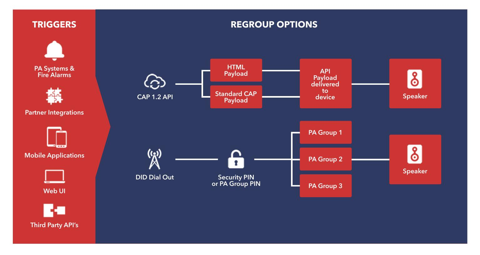
Newer Simplex Fire Panel Models can trigger or receive real-time alerts from Regroup using direct FEMA standard CAP 1.2 APIs.
